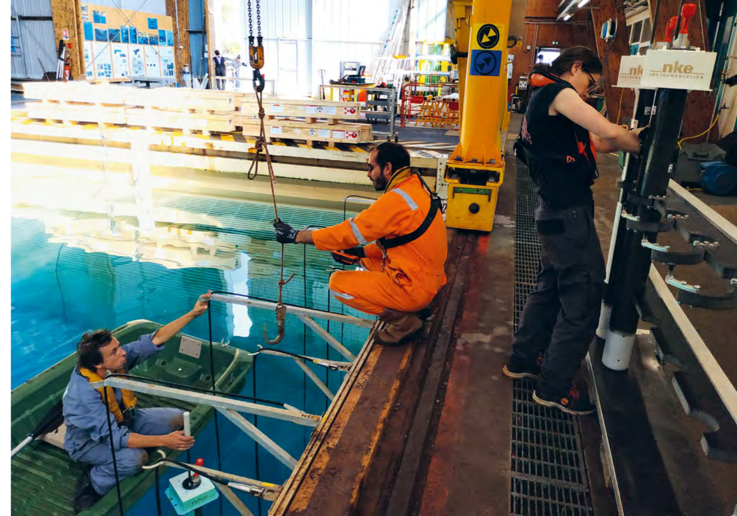
Testing the Deep Argo CTS4 floats at the test basin in Brest.
