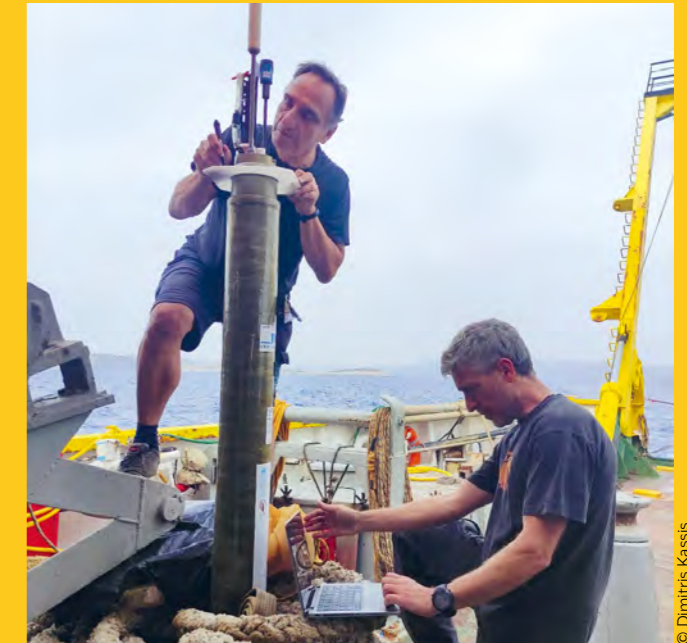
Pre-deployment testing of a Deep Arvor-I float in the Ionian Sea.
